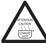
Avoid touching the cabinet surfaces which may have temperatures over 170° F. (77° C) Use caution when opening either door due to steam exiting out.
