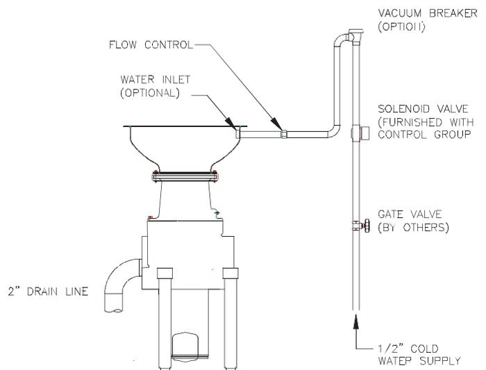
4. All controls are supplied with a solenoid valve which must be installed in the water supply line as shown.
