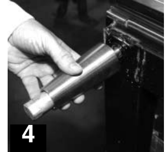
4 Thread leg into cabinet bottom frame rail.
